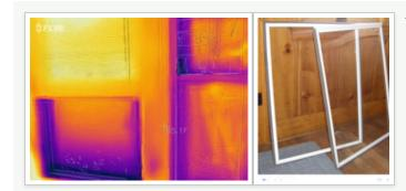
This is an infrared photo of a typical window with a cellular window treatment warming the top window .Use window treatments or interior storms to insulate your windows.
