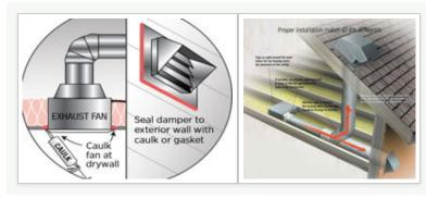
Moisture Control: Bath and kitchen venting should be in an insulated duct connected to a flapper venting directly outside. This will reduce moisture in the home and into the attic space.
