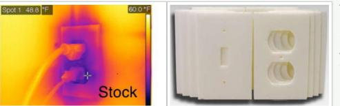
Typical Air Leakage at Electrical Outlet, on exterior walls: Outlet gaskets go behind switch and wall plates to stop heat loss.
