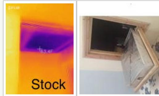
Typically an uninsulated attic hatch is one of the biggest leaks in a home. Insulate the hatch to your attic or crawl space.
