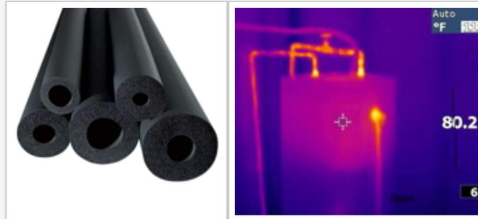
Foam sleeve type insulation works well on water heating pipes. The first 6 to 10 feet closest to the water heater provide the most benefit to insulate.
